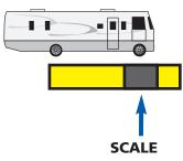
The RV must remain as level as possible on the scale (even when an axle or side isn't on the scale). Therefore, to obtain side-to-side weights, there must be enough space on either side of the scale to accommodate the RV being partially off the scale.
