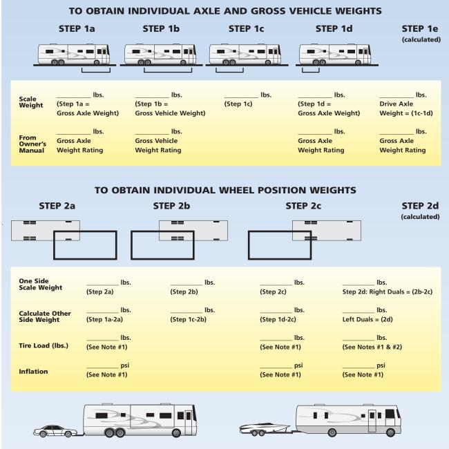
1. From the tire manufacturer's load and inflation tables or the sidewall of the tires mounted on the vehicle. 2. If vehicle has duals, read dual capacity from tire and multiply by 2 to obtain dual assembly load capacity.
